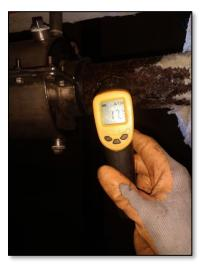
Measure pipeline temperature during the entire pipe freezing process
